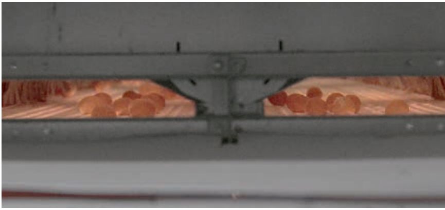
Two divided longitudinal egg belts transport the eggs securely
